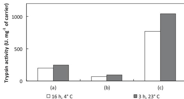
Figure 4. Proteolytic activity of magnetic Tryp-PGMA-COOH microspheres under various reaction conditions (time, temperature, and presence of EDC and sulfo-NHS). (a) One-, (b) two-step protocol with EDC, and (c) one-step immobilization with EDC and sulfo-NHS.
