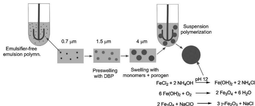
**Scheme 2.** Preparation of monodisperse magnetic macroporous polymer microspheres by multi-step swelling and polymerization method and precipitation of iron oxide inside their pores.
