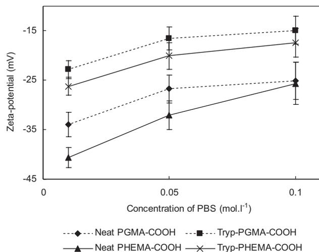
**Figure 7.** Zeta-potential of magnetic PGMA-COOH and magnetic PHEMA-COOH microspheres before and after biofunctionalization with trypsin in phosphate buffer (pH = 7.3); activity  $970 \text{ U} \cdot \text{mg}^{-1}$  of Tryp-PGMA-COOH and  $1417 \text{ U} \cdot \text{mg}^{-1}$  of Tryp-PHEMA-COOH.
